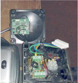
If the lid is in the way then the white multi pin plug can be pulled off to separate the lid from the body.
